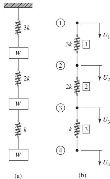
**Figure 2.4** Example 2.2: elastic spring supporting weights.
