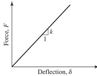
**Figure 2.8** Force-deflection relation for a linear elastic spring.
