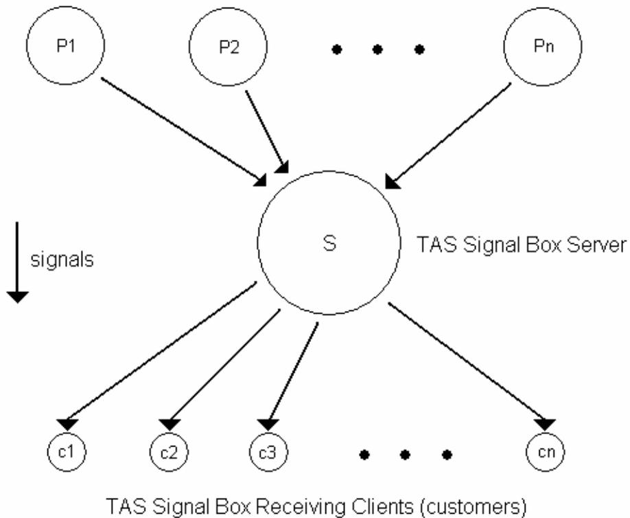
Signals generated from the posting clients, pass through the server and on to the end-user client applications
